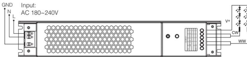
Controller connect to color temperature LED strip diagram
