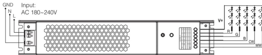
Controller connect to RGB+CCT LED strip diagram
