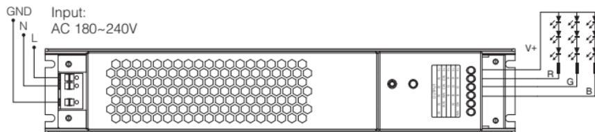
Controller connect to RGB LED strip diagram
