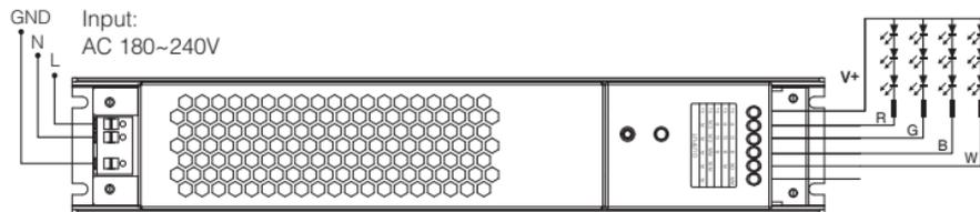
Controller connect to RGBW LED strip diagram
